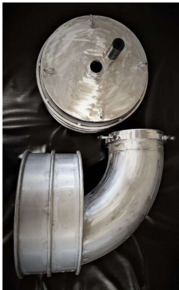
Image: Example of WIP bend and packer
